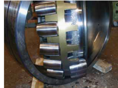
Figure 17. Spherical bearing in Valmet shop.
