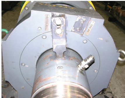
Figure 16. New style of shaft locking key in place on a roll.
