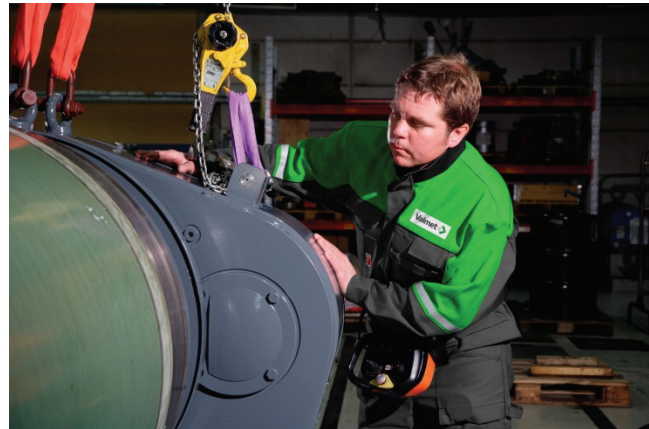
Figure 1. Valmet's experts reconditioning a deflection compensated roll at a roll shop.
